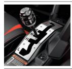
The shift plate is made from durable stainless steel and bolts into place for a secure fit.
